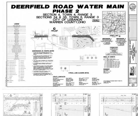
Communication between field crews and office staff was critical for the Deerfield Road water main. Bayer Becker provided design on the 16" ductile iron water transmission main for the City of Lebanon. The project consisted of two sections, a 1,100 linear feet section between W. Turtlecreek-Union Road and the State Route 48 ramp and a 2,170 linear feet section located between Navaho Drive and Cook Road.
